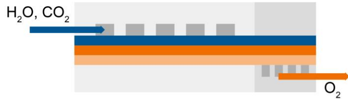
Simplified figure of SOEC cell structure
